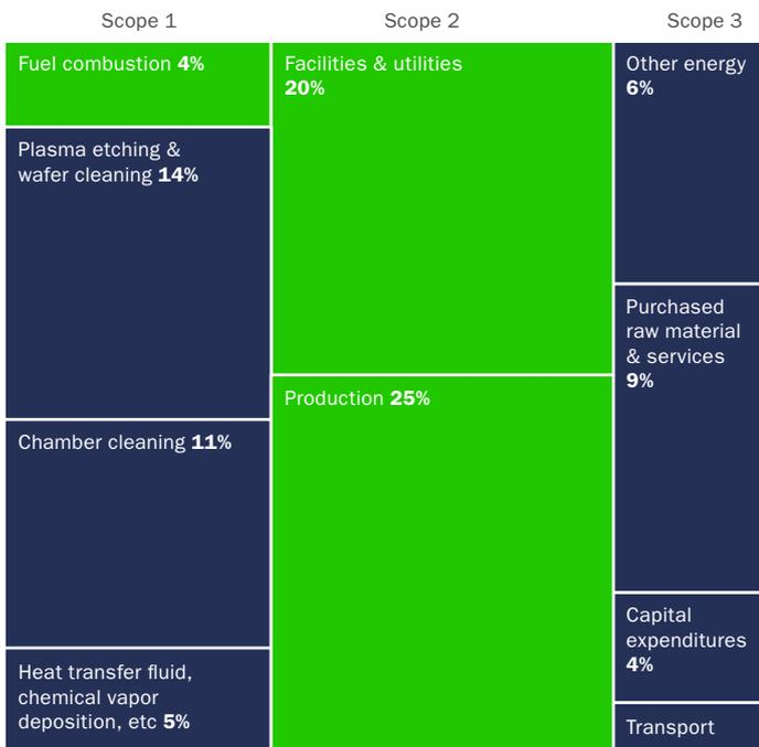
Notes: 1. Green indicates areas where most emissions are CO<sub>2</sub> and can be reduced by switching to renewable energy; 2. Scope 3 downstream are excluded. Sources: Authors’ analysis aggregating data from a) McKinsey 2022, and b) US EPA GHGRP.
