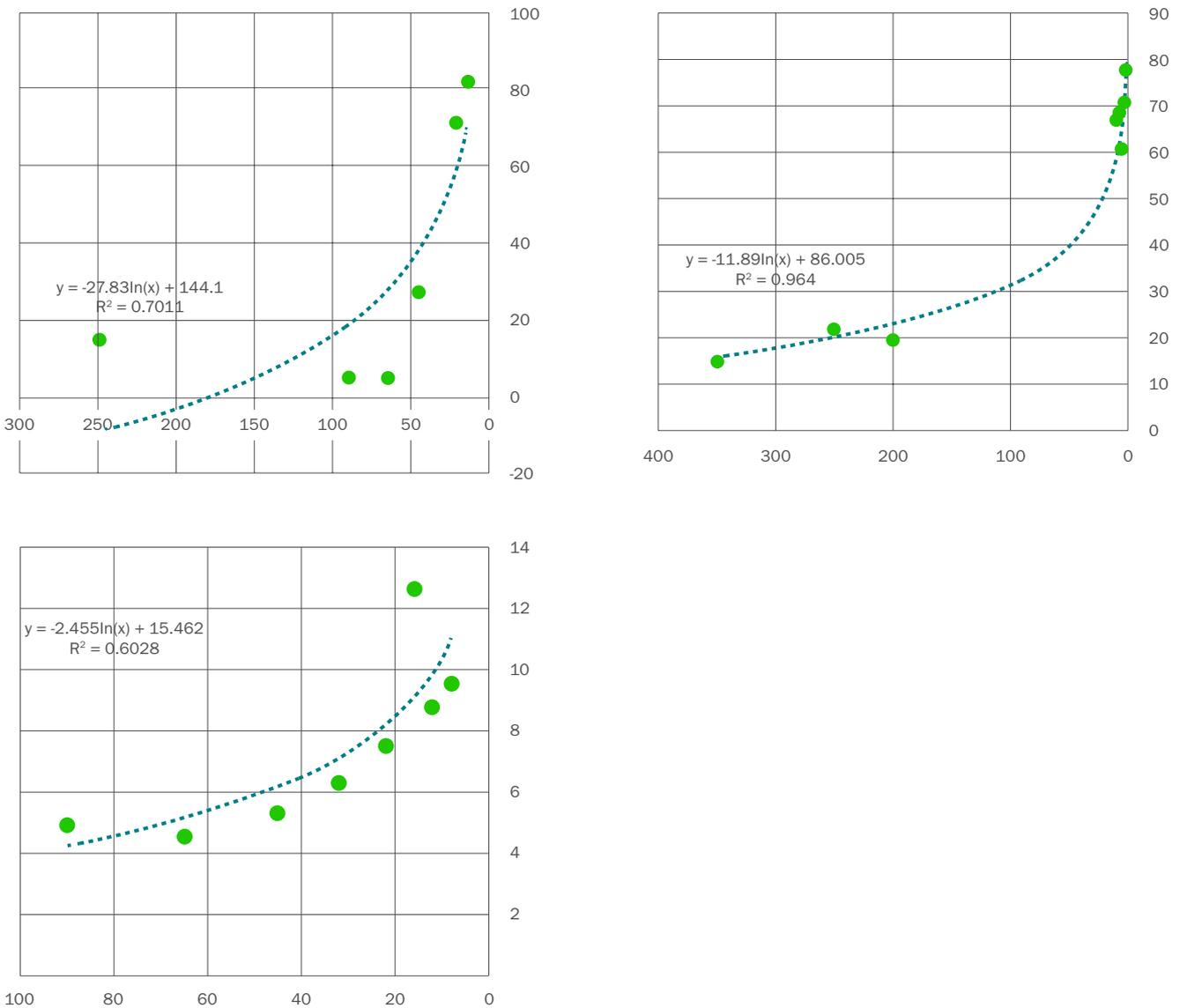
Notes: X-axes are all reversed node sizes ranging from 350nm to 3nm; Y-axes are different, from left to right, electricity intensity, mask count, and turnaround time, respectively.<sup>20</sup>
